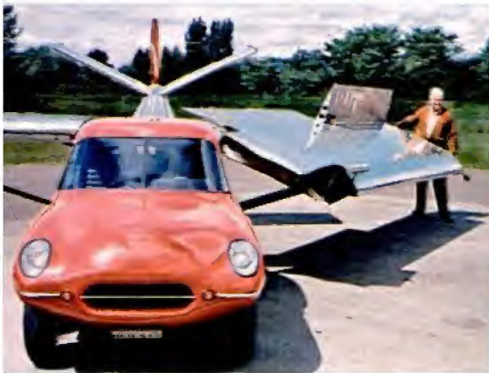
BUG BECOMES BIRD as two pins are driven in place to secure flight component and wings unfold for takeoff
